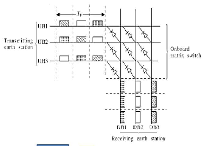
SS-TDMA concept used in INTELSAT-VI.
